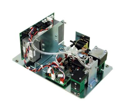
Sensors' Standard Emissions Module is complete with the Sensors AMBII Microbench, a carefully selected pump and filtering system, a customized 12-volt power supply and driver p.c. board - prepared for the supply from a vehicle's battery - and a chassis for easy incorporation into a gas analyzer housing.
